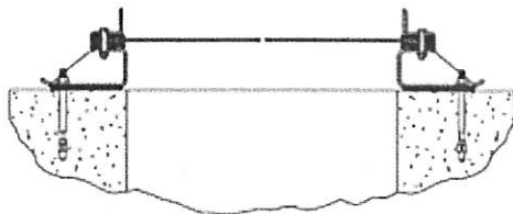
Figure 20-02 Directly mounted on a concrete wall (CW)
